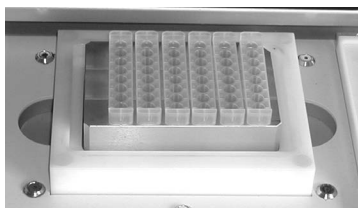
Figure 5: NucleoSpin® Plasmid Binding Strips inserted into Column Holder D placed in the manifold bottom on the Qiagen BioRobot® 9600.
