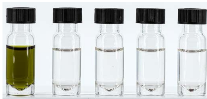
Figure 4: Visible matrix reduction: cannabis extract, competitor 1, competitor 2, competitor 3, MACHEREY-NAGEL (from left to right).
