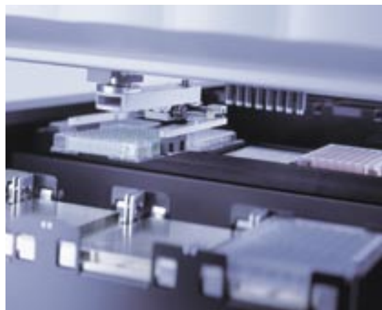
Figure 2: The internal plate handler iSWAP can also reach positions outside of the MICROLAB® STAR deck.
