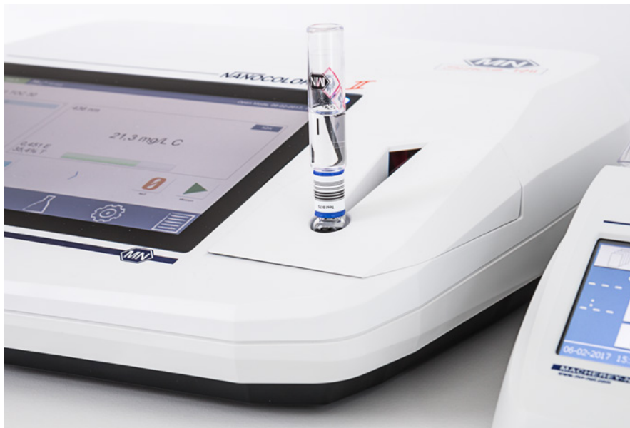
Quantitative determination of the generated CO 2 by an indicator (reaction basis analog to DIN EN 1484)
