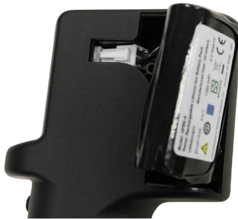
4. Push down on connector latch and pull battery loose from the board.
