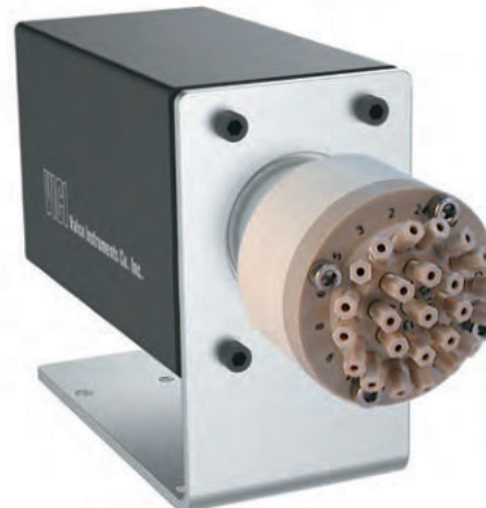
24 POSITION SELECTOR 1/16" 6-40 PEEK fittings
