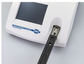
Pic. 17: Reinsertion of the test strip holder
