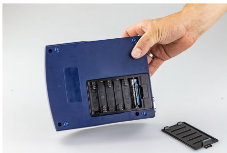
Pic. 15: Battery compartment
