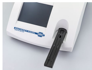
Pic. 18: Check alignment of notches
