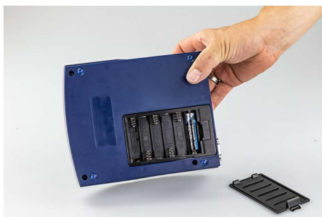
Pic 17: Battery compartment
