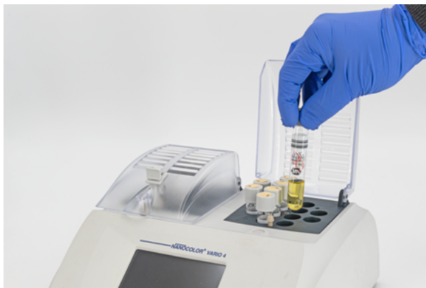
Figure 15: Inserting cuvettes into the heating block
