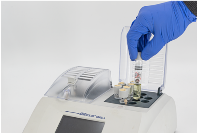
Figure 17: Removing the cuvettes from the heating block
