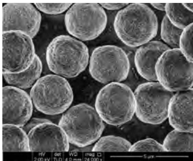
Electron microscopic image of NUCLEOSHELL®
