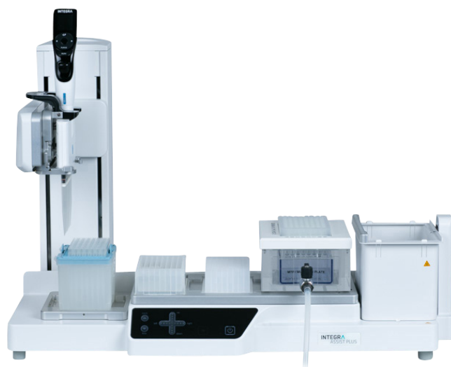
Figure 1: General set-up of the ASSIST PLUS pipetting robot for the tissue DNA isolation program.
