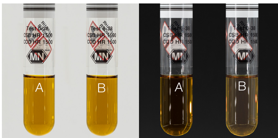
2 cuvettes (A | B) with the same COD concentration. The turbidity in cuvette B influences the result by up to 30 %.
