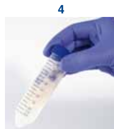
Blue LyseControl still visible – continue inverting
