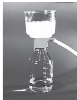
Figure 3: Correct use of the NucleoBond® Bottle Top Filter
