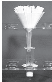
Figure 2: Correct use of the NucleoBond® Folded Filter, NucleoBond® Column placed in a Plastic Washer
