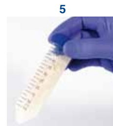
LyseControl completely colorless – sufficient inverting
