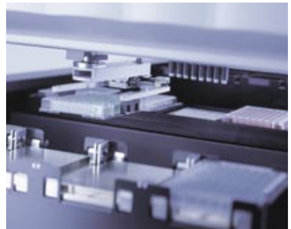
Figure 2: The internal plate handler iSWAP can also reach positions outside of the MICROLAB® STAR deck.
